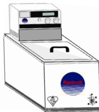
Heater/Bath Circulator Pump
